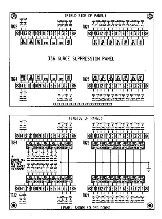
For base mounted cabinets, mount surge protection panels on the left side of the cabinet as viewed from the rear. Attach each panel to the cabinet rack assembly using bolts and make it easily removable. Mount the surge protection devices in vertical rows on each panel and connect the
